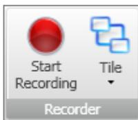
The **Recorder** section of the ribbon bar contains a **Start Recording** button that launches the Recording Surface side-by-side with WebUI. The **Tile** button can place the Recording Surface on the left or right of the WebUI window.
