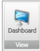
The **View** section of the ribbon bar contains only the **Dashboard** button. Toggling the Dashboard button on allows you to get a snapshot view of all your testing activity at one time.
