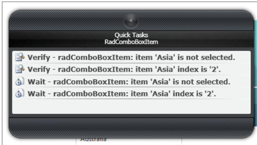
The State verification for a RadComboBox item has all the possible values in the drop down and also lets you test if a particular item is Selected, Visible, Enabled or Highlighted.
